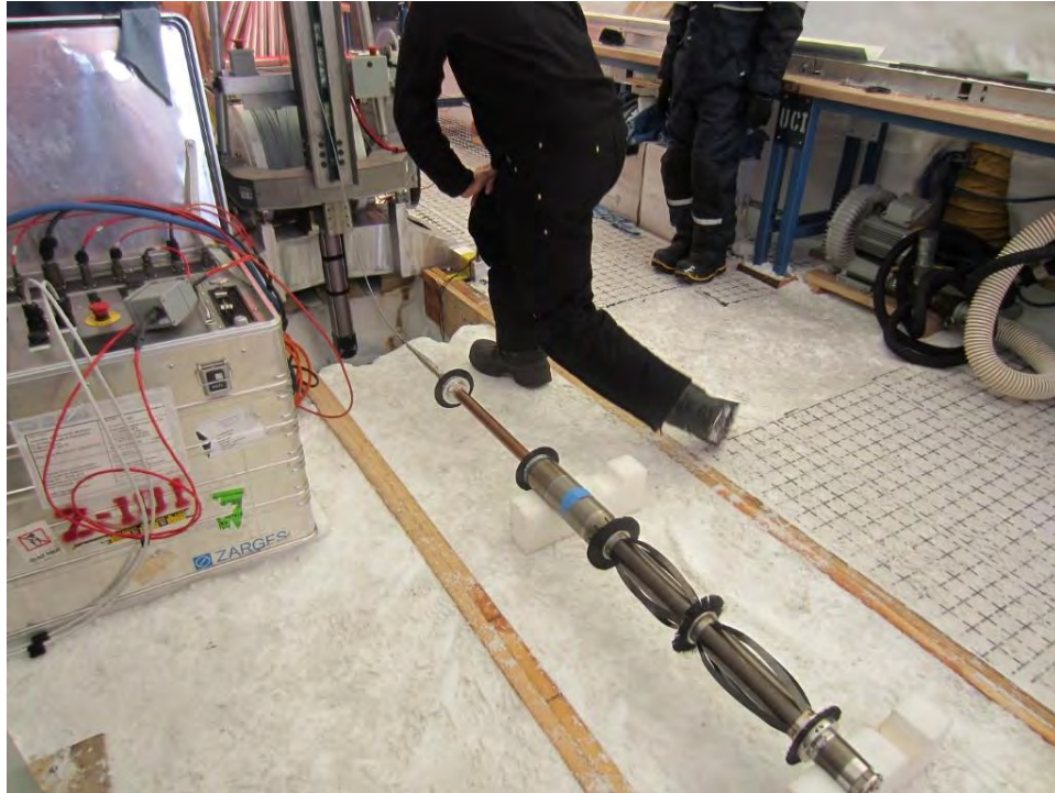
Dust logging tool being tested on the logging winch cable
